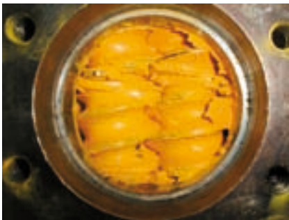
ContiMixer in operation: pre-dispersing of offset inks.
