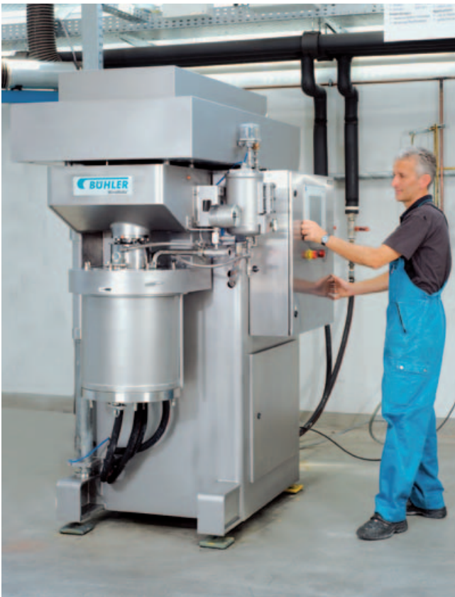
Fig. 7.3: MicroMedia™ P3 – production size mill (stainless steel version) for micro beads, with additional rotor cooling.
