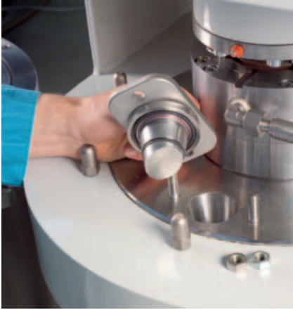
Fig. 11.1: Double-sealed plug for closing of filling and discharge opening for micro beads.
