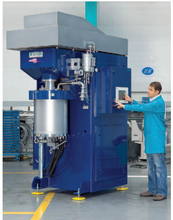
Fig. 7.4: MicroMedia™ in customer finish, nano processing in the mass production with an installed power of P = 90 kW. Cleaning of inner surface of MicroScreen during operation by means of an in-situ device.
