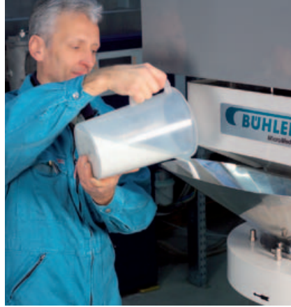
Fig. 11.2: Firmly attachable, sealed special device for filling of micro beads.
