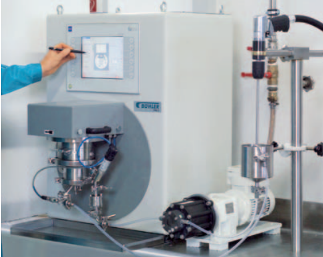
Fig. 7.1: MicroMedia™ L (active chamber volume 0.07 l = 70 cm 3 ) with recirculation set-up in the development lab, mounted to the universal Lab Perl Mill™ PML 2.
