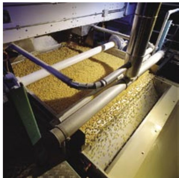
A computer program checks the depth of product based on the product recipe or shape.
