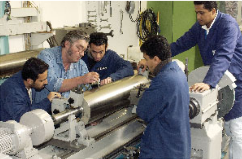
Optimal corrugating of rolls. Training on the grinding and corrugating machine of the Training Center ensures optimal roll corrugations (flutes).
